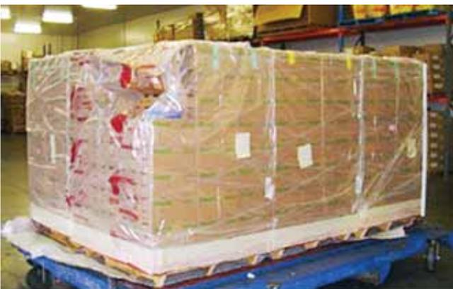
Skids are placed onto a PMC ULD and flown to Australia. The ULDs are completely insulated with foil and then frozen gel packs are placed onto the skids to maintain temperature.
